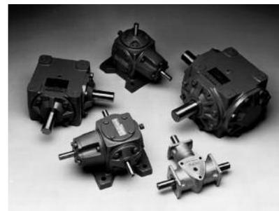
**Right-angle gear drives** are available with single or double output shafts and are designed for high capacity and efficiency, quiet operation, and long service life. Bevel or spiral bevel gears are made of hardened alloy steel, with oversized bearings and high-quality oil seals.
