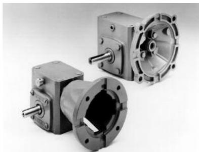
**700 Series single-reduction** worm gear speed reducers feature integral hardened worms and bronze worm gears. Through-bore housings assure true shaft positioning, proper mating of worm and gear, and perfect alignment under maximum stress conditions. Oversize roller and ball bearings allow greater overhung and thrust loads.
