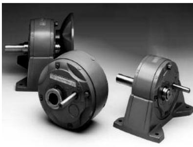
**200 Optimount Series** helical gear speed reducers contain gears and pinions made of heat-treated alloy steel or close-grain cast iron, with ball or tapered roller bearings. Rugged housings are precision-machined to assure accurate and permanent gear alignment.
