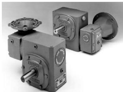
**W700 Series double-reduction** worm gear speed reducers offer a broad range of reduction ratios, with integral hardened worms and bronze worm gears used throughout. Mounting surfaces are machined parallel for correct alignment of all drive components. Precision through-bore housings assure true shaft positioning with proper mating of worms and gears.
